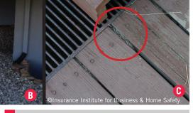
A Embers that pass through deck board gaps will land on the ground, or on combustible materials stored under the deck, as shown during this IBHS test.
