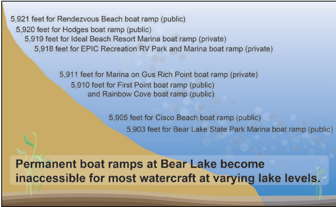
Figure 2-50. Lake level effects on boat ramps in the planning area.
